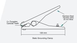
ATEX certified / FM Approved 2 Pole stainless steel grounding clamp fitted with one pair of tungsten carbide teeth.
