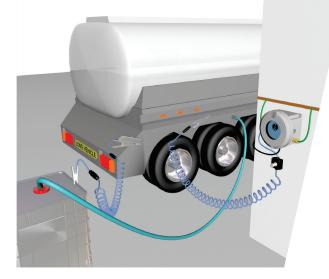
Example of grounded truck bonded to IBC
