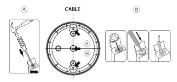
In order to ensure the luminaire is sealed, it is vital to use the cable grommets.
