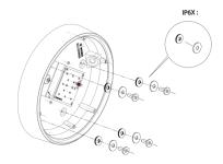
For mounting the luminaire, use 5 mm diameter flatheaded screws with fixing plugs suitable for the type of wall, in order to achieve optimum rip-out resistance. The screws and plugs are not supplied with the luminaire.
