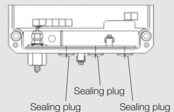
Sealing plug      Sealing plug      Sealing plug
