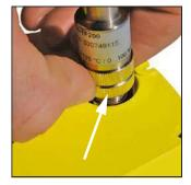
For mounting the sensor must be plugged into the socket and screwed on the sensor by turning the lower knurled screw clockwise. Tighten hand-screwed only.
