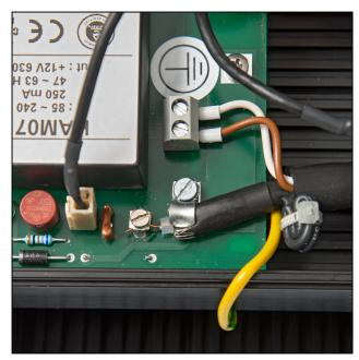
Attaching the cable in the terminal box
